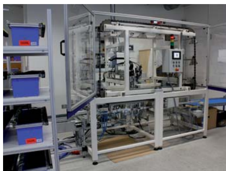
Automated filling of 2K-epoxy resin at the moulding station
