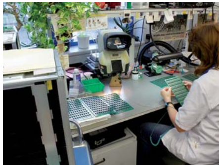
Quality Assurance QA-visual inspection of the circuit boards
