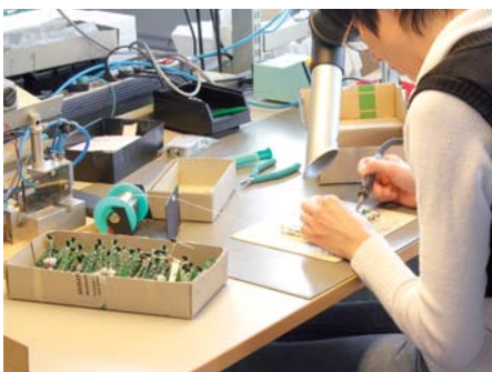
Sensor assembly with QA-function-test
