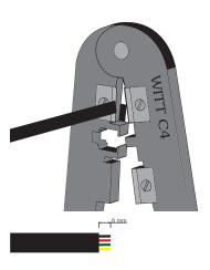
3. Arrange the cable in the color sequence shown and insert into the correctly positioned plug
